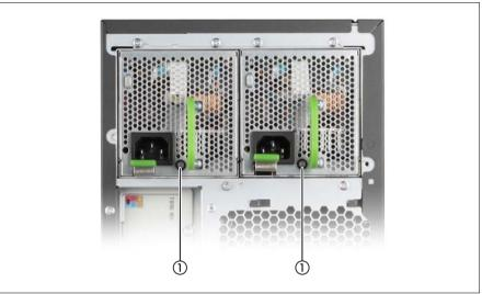
Figure 19: Indicators on the hot-plug power supply units
